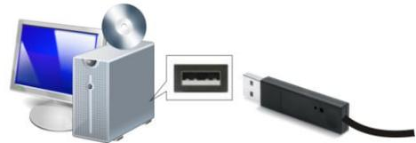
3. Connect the standard-sized connector on the USB cable to a USB port on a second computer.
